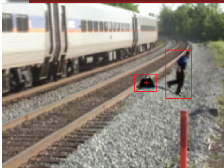
Top, camera captures man walking along Amtrak rail bed parallel to the moving train. Center, ObjectVideo VEW detects man as potential threat. Bottom, when man leaves bag, an alert is issued to security personnel. Courtesy ObjectVideo
